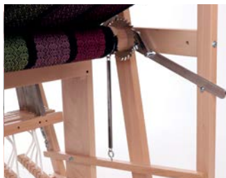
Easy action warp advancement with steel ratchet
