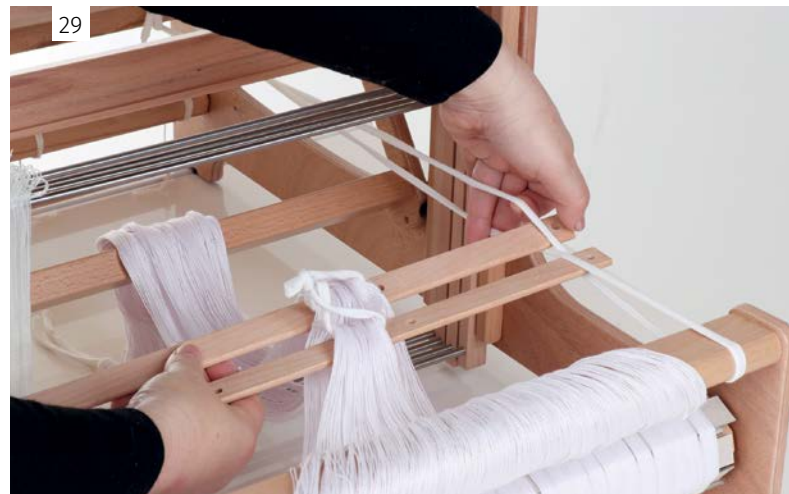
29 To support the cross sticks, use the helping hands, crossed in a figure eight.
