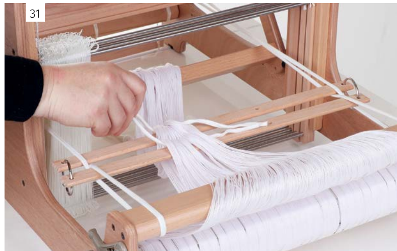
31 Remove the threading cross tie.
