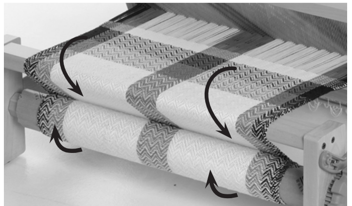
Winding the warp on the front roller.
