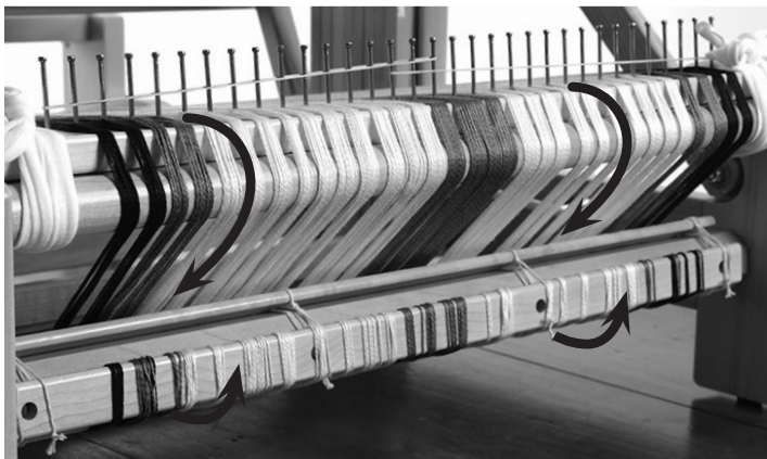
Winding the warp on the back roller.
