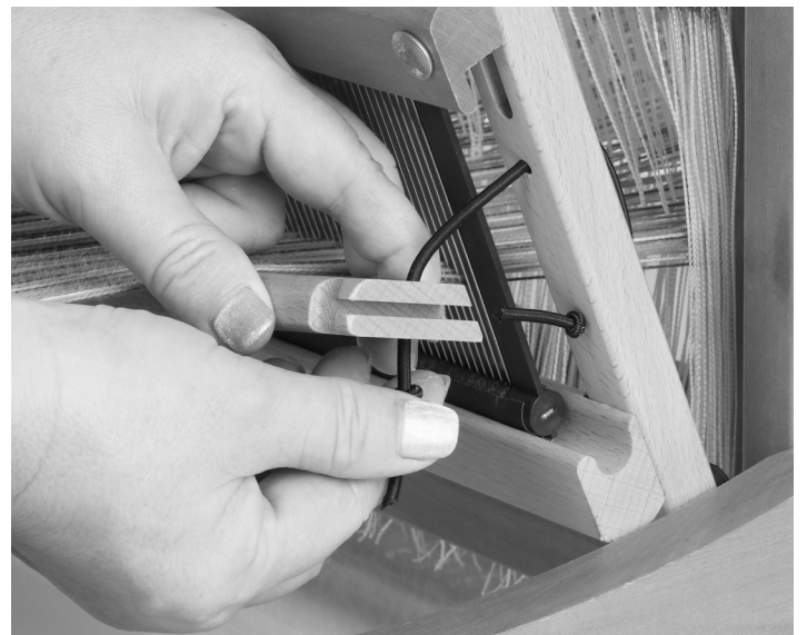
14. Then down through the hole in the Shuttle Race and tie a knot loosely (so it can be adjusted).
