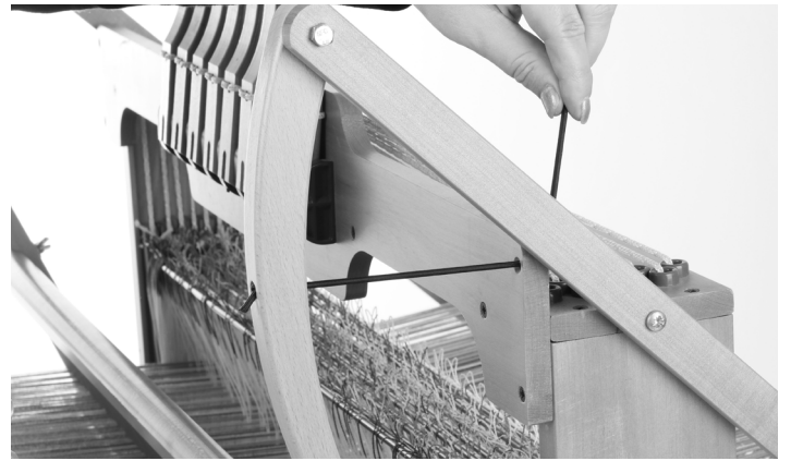
11. Tie a knot in one end of the stretchy cords, feed them through the top holes in the beater arms, through the holes in the castle front and tie a knot. Adjust the position of the knots to increase or reduce the tension so the rubber feet touch the castle sides.
