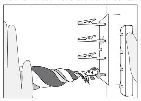
4. Holding onto the ends, unclip and place all 4 opposite ends into one clip and rotate anticlockwise.
