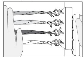
3. Place a hand on the ends of the sliver and rotate the handle clockwise until the sliver is twisted.
